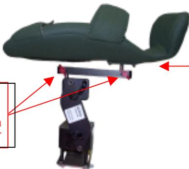
7. Adjust the **RED wing bolts** to control lateral and Pivot movement after the desired vertical position is reached. **TO LOCK** the Lateral-Pivot movement, loosen the **RED wing bolts** and tighten the small **Silver screws** with finger or Allen wrench provided; then, Re-tighten **RED wing bolts**.
